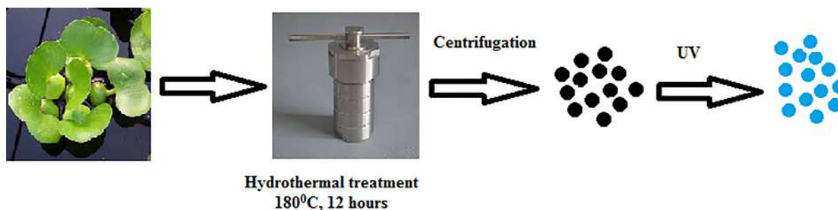
Fig. 1. Scheme for the synthesis of photoluminescent N-CDs by hydrothermal treatment of water hyacinth.
